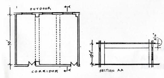
**Design f:** Gypsum Board being expensive, it may be advisable to apply locally available Partex on a suspended ceiling, the rear wall and the wall opposite to the windows. The absorption will be  $\{(1080+292.5) * 0.25\} = 343.13$
